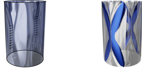
Figure 6: Cylinder with top and bottom nodes fixed and pulling force (100N) distributed on two sides. Left: the initial deformation before topology optimization with boundary condition marked in black. Right: the optimized structure.
