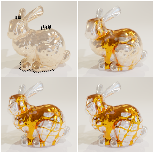
Figure 12: Optimization intermediate states of the Stanford bunny at iteration 1, 20, 100 and 250. The boundary condition is indicated in the first picture, where the bottom nodes of the bunny are fixed and loads are applied on the head and the back.
